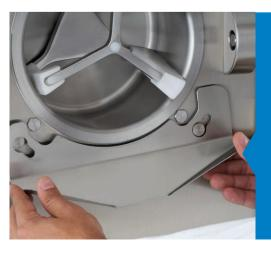
Cleaning is easy thanks to **hot** washing of the cylinder and the removable gelato extraction chute.
